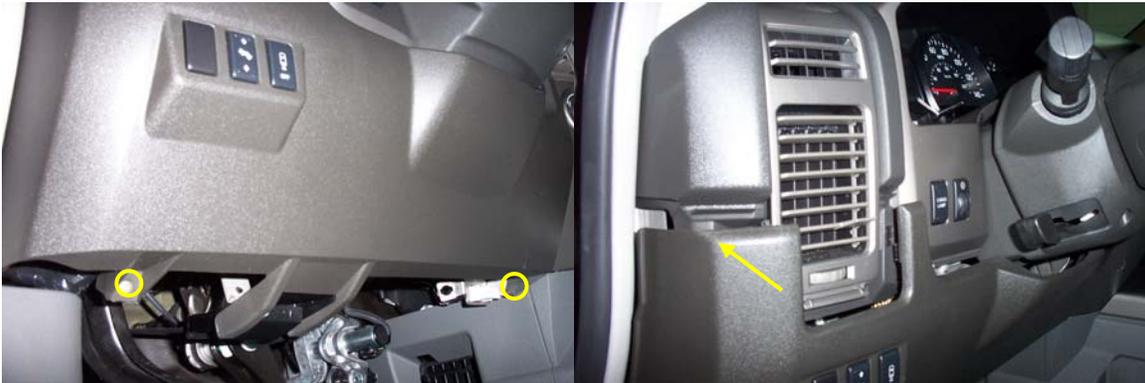
4. If the truck's gear selector is is not on the column, skip this section and proceed to section 5. However, if the gear selector is on the column, it helps to disconnect the gear selector when removing the Upper Instrument Panel Bezel.
