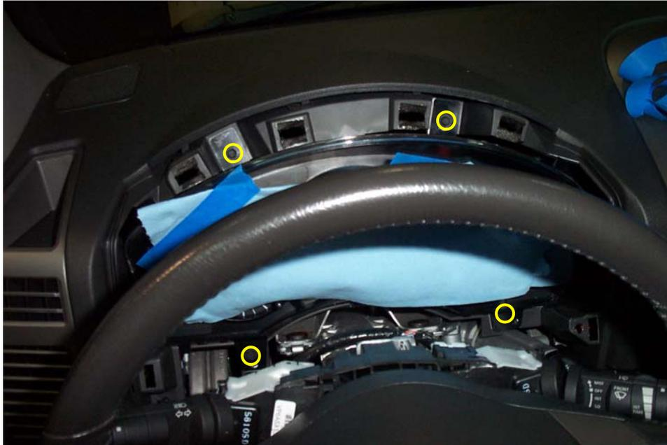
7. Disconnect the factory cable from the Instrument Panel. Press the release mechanism, and gently pull straight. To prevent damage, do not rock the connector.
