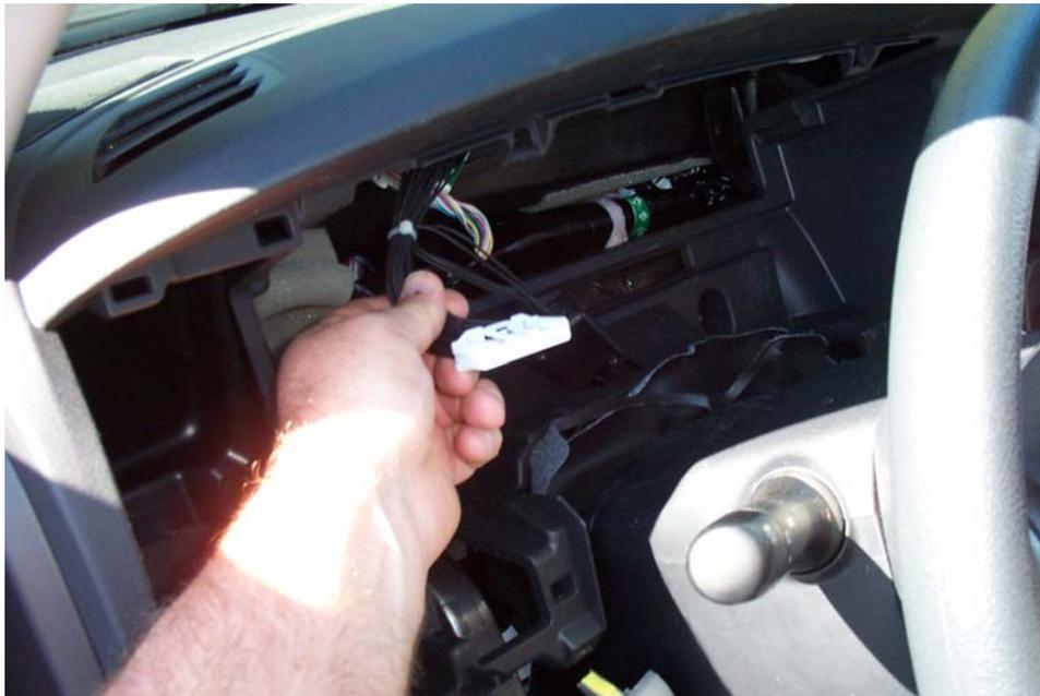
14. Reverse the process of this document to properly re-install the Instrument Panel components.
