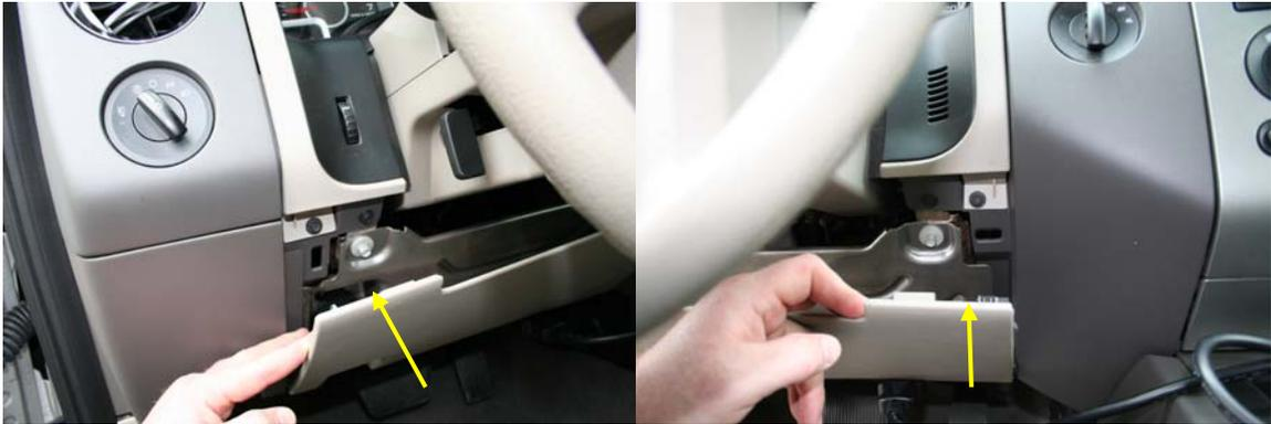
4. Remove the Upper Instrument Panel Bezel
