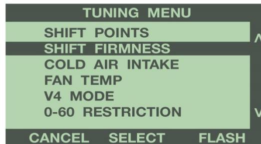
Some vehicles have only one pre-determined setting for shift firmness, and will not have a selectable adjustment. If your vehicle has this setting, the programmer will display a Yes or No option. Highlight the desired choice, and press 'Select'. Some vehicles have the option to select between 25%, 50%, 75%, and 100% for the level in which to enhance shifting firmness.
