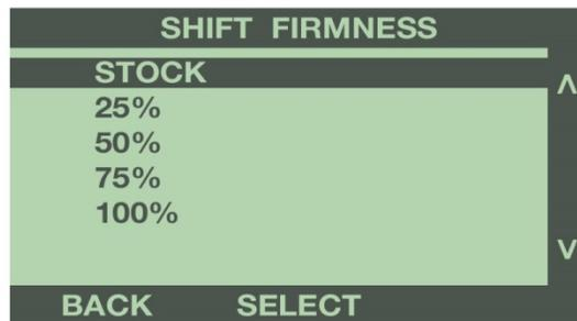
Press the 'Back' button to go back to the Gear Shift menu. Repeat the procedure above for each gear change. Once you have made the desired changes for each gear, press the 'Back' button to return to the Tuning Menu. For more information on Shift Firmness option, see Programming Features explanation in Section 4.
