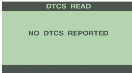
If the vehicle has any DTC’s, the programmer will display all DTC’s, and the total number of DTC’s reported from the vehicle’s computer. To clear all DTC’s, press the ‘Clear’ button. To see a definition of each DTC, press the ‘More’ button.
