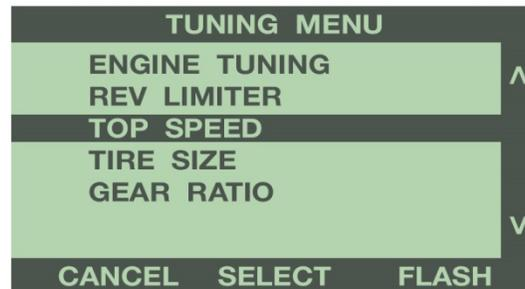
Use the buttons to the right of the screen to scroll up or down, and highlight the desired MPH. Press ‘Select’ to save the chosen value.
