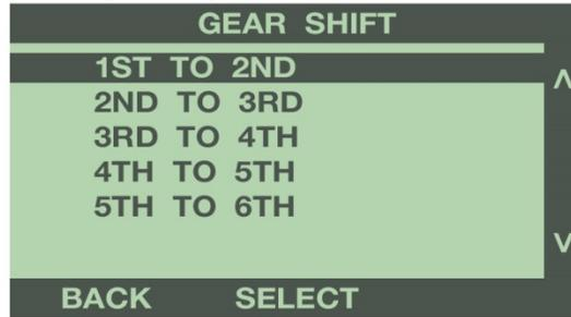
Press the 'Select' button, then use the buttons to the right of the screen to scroll up or down, and highlight the value to increase or decrease the shift points, in 100 RPM increments. Press Select to save the chosen value.
