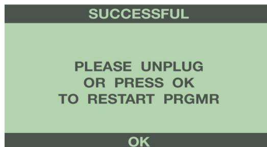
It is now safe to unplug the programmer from the vehicle and start the engine. Make sure the “Check Engine” light on the instrument cluster goes out (If it stays on or flashes, read out the DTC’s, and contact Hypertech tech support). Warm up the engine and make sure it is running smoothly.
