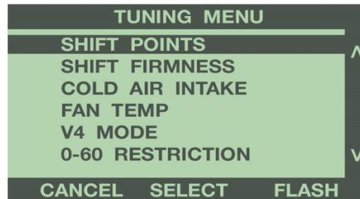
To adjust the shift points in all gears the same, select ALL from the Shift Points menu. To adjust the shift points for each gear change separately, select PER GEAR from the Shift Points menu.
