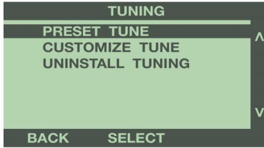
When using the programmer for the first time, select the **CUSTOMIZE TUNE** option.
