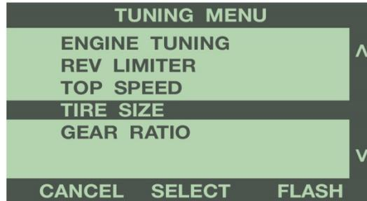
Use the buttons to the right of the screen to scroll up or down, and highlight the desired tire size, in ¼ inch increments. Press 'Select' to save the chosen value.
