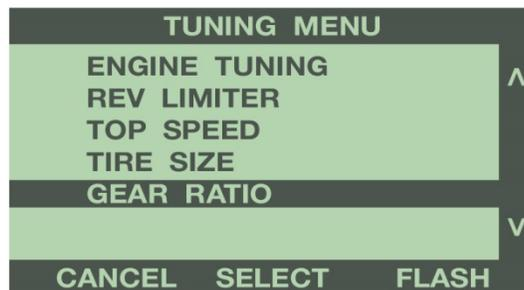
Use the buttons to the right of the screen to scroll up or down, and highlight the desired ratio. Press 'Select' to save the chosen value.
