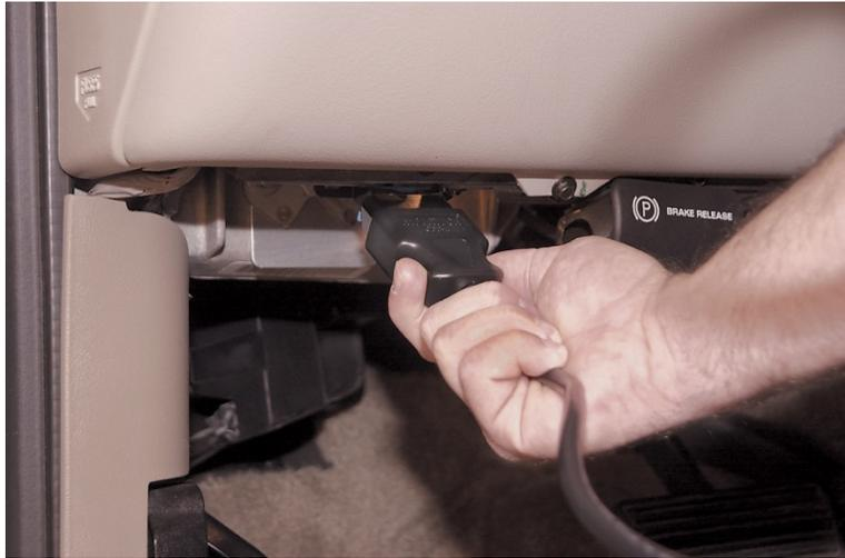
Make sure the cable is plugged in completely to ensure a good connection. **DO NOT disturb the cable once it is connected to the diagnostic port.** The programmer will power up, and display the startup screen.
