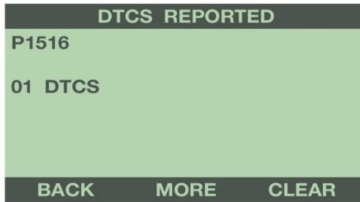
Use the buttons to the right of the screen to scroll up or down and review each DTC. The programmer will display a description of the DTC.
