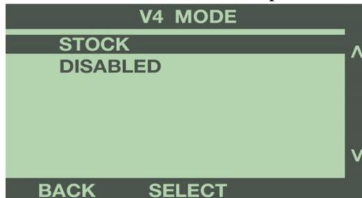
To adjust the minimum speed that the V4 Mode turns off, use the buttons to the right of the screen to scroll up or down, and highlight the desired speed. Press the 'Select' button to save this option.
