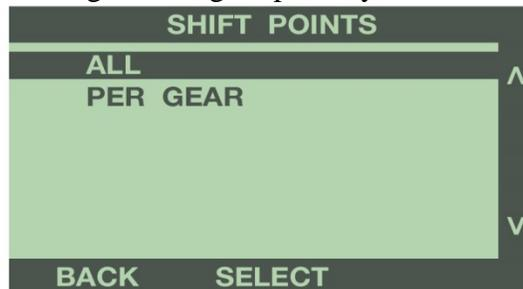
**ALL SHIFT POINTS:** Use the buttons to the right of the screen to scroll up or down, and highlight the value to increase or decrease the shift points, in 100 RPM increments. Press ‘Select’ to save the chosen value.
