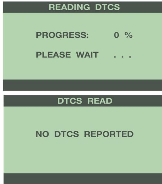
If the vehicle has any DTC's, the programmer will display the number of DTC's reported from the vehicle's computer. You can review the DTC's by pressing the 'Show' button. Before the programming process can begin, all DTC's must be cleared. To clear any DTC's, press the 'Clear' button. For more information on this feature, see the DTC section. Once the DTC's are cleared, the programmer will proceed to Reading Vehicle.
