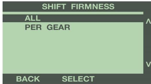
**ALL SHIFT FIRMNESS:** Use the buttons to the right of the screen to scroll up or down, and highlight the percentage to increase or decrease the shift firmness. Press Select to save the chosen value.
