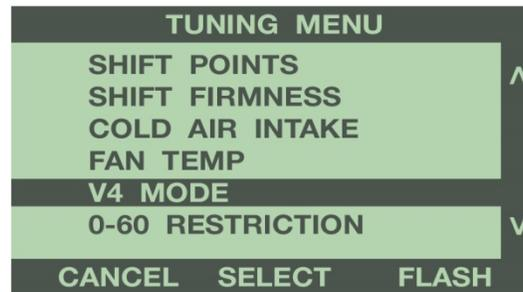
To completely disable the V4 Mode, use the buttons to the right of the screen to scroll down, and highlight Disabled. Press the 'Select' button to save this option.
