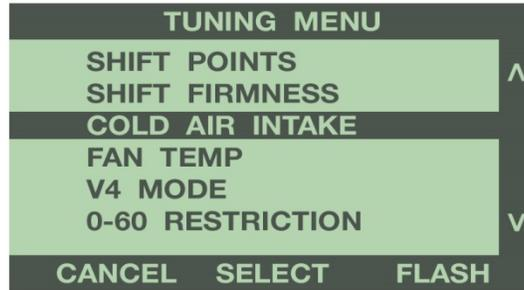
Use the buttons to the right of the screen to highlight the cold air intake installed on your vehicle. Select the Stock air intake if you have not installed an aftermarket air intake. Press 'Select' to save the chosen tune.
