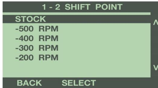
Press the 'Back' button to go back to the Gear Shift menu. Repeat the procedure above for each gear change. Once you have made the desired changes for each gear, press the 'Back' button to return to the Tuning Menu. For more information on Shift Points options, see Programming Features explanation in section 4.
