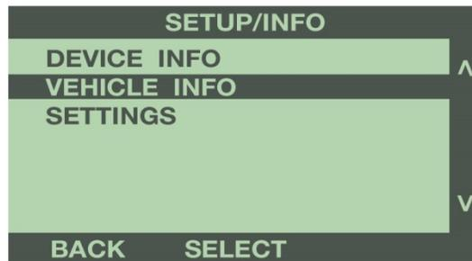
The Vehicle Info menu displays the VIN number of the vehicle that the programmer was last connected to, and the current status of the programmer.
