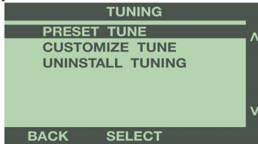
Use the buttons to the right of the screen to highlight a Preset Tune, and press 'Select'.
