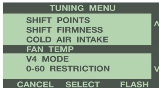
Use the buttons to the right of the screen to scroll up or down, and highlight the temperature to turn on the cooling fan. Press 'Select' to save the chosen value.
