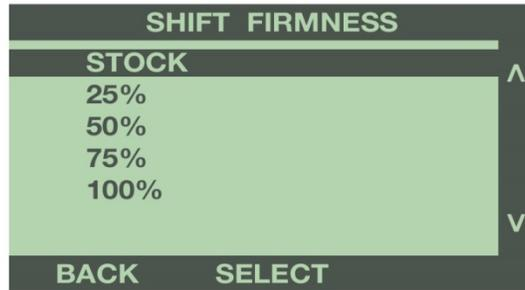
**PER GEAR SHIFT FIRMNESS:** Use the buttons to the right of the screen to scroll up or down, and highlight the gear change to adjust.
