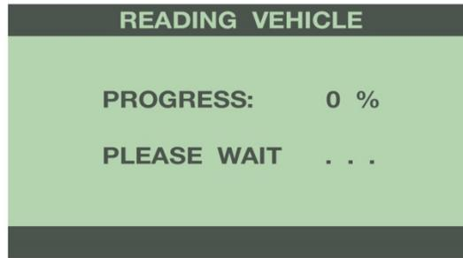
Once the programmer has completed the reading process, it will proceed to the Writing Vehicle mode. Continue to follow the messages on the screen. You may be prompted to turn the key to the 'RUN' and 'OFF' position during this process.
