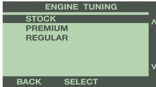
Press 'Select' to save the chosen tune. By selecting 'Stock', the programmer will install any additional features selected, but keep the stock engine tuning. For more information on Gas Engine Tuning options, see Programmer Features explanation in Section 4.
