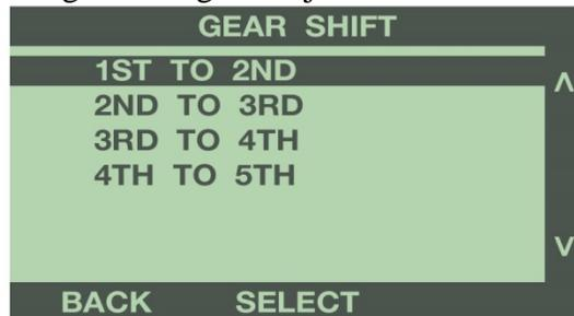
Press the 'Select' button, then use the buttons to the right of the screen to scroll up or down, and highlight the percentage to increase or decrease the shift firmness. Press 'Select' to save the chosen value.
