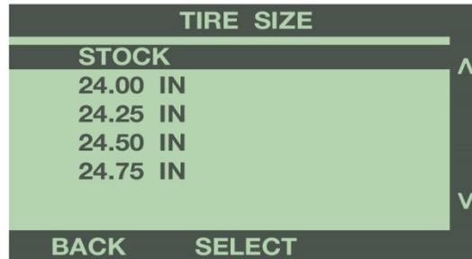
**Note: Only select this feature if the vehicle has a different size tire than what was installed from the factory.** For more information, see Programming Features explanation in Section 4.
